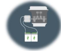
All four electric vehicle types use regenerative braking to charge the battery. While braking, the motor is still spinning even though the car is trying to slow down.
